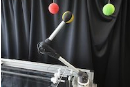
Figure 1.6: Muscle-based robotic arm serving as a testbed for Learning for Control. While it offers unique possibilities in terms of high accelerations, extreme speeds, and variable stiffness actuation, classical control methods are unable to unlock these abilities.
