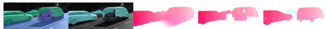
Figure 7: Failure case. From left to right: Initial segmentation; SOF segmentation; Flow estimation from DiscreteFlow; Flow estimation from SOF; Ground truth flow. Our layered method assumes two dominant motions in the region, failing if there are more than two motions.
