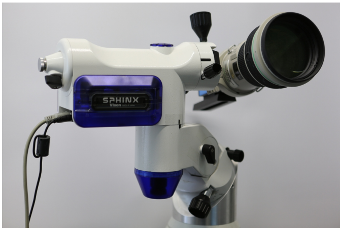
Fig. 8. The telescope mount used for the tracking experiments. On the right side is the camera lens used as guiding telescope. A main telescope is not used for the tests.
